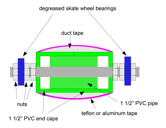
Nuts lock the roller and bearings into position on the threaded rod. Bearings are locked into main PVC pipe by screws.
